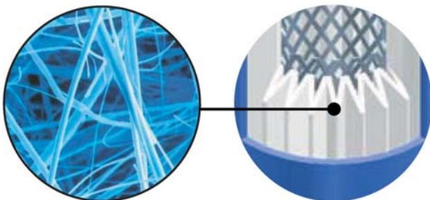
**Cross section of the depth filter
